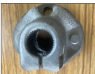
Two different C2 flange castings with different numbers of splines C2 Copper ground straps
