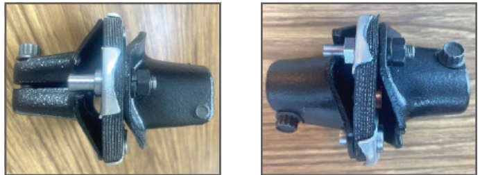
1963-1966 Steering Coupling with Non-Telescoping steering shafts. Note bolt head (round and hex) extending through slot in casting.
